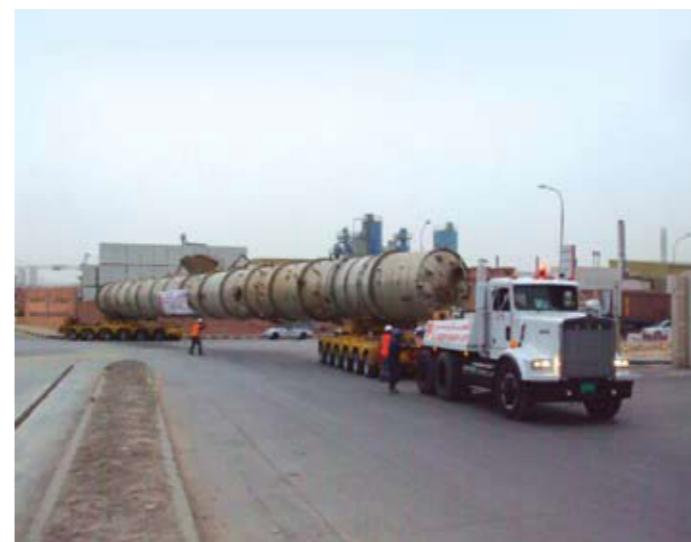
Transportation of a 43 meter long vessel (above) using 24 axles of conventional hydraulic trailers in the Kingdom of Saudi Arabia.
