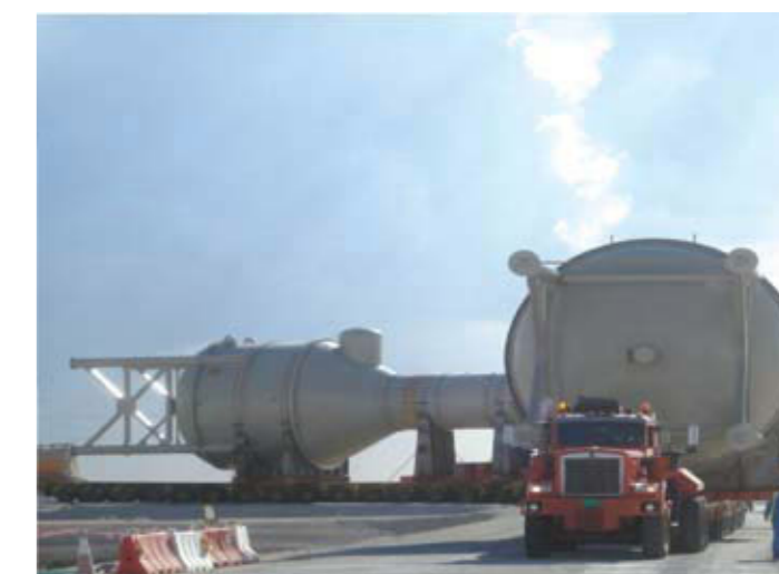
Transportation of a 240 te brine evaporator (above) utilising 24 axles of conventional hydraulic trailers in Qatar.
